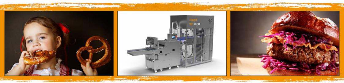
The automatic loader (WP Automatic Loader) opens up a new dimension in lye application. An hourly throughput of approx. 240 trays per hour can be achieved with less labour. This means you can achieve far greater efficiency.
