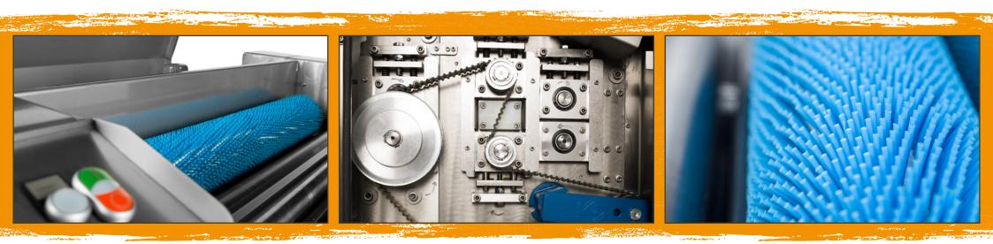
The BRM Deluxe is an advanced tray cleaning system specially developed for the hygienic cleaning and greasing of baking and perforated trays.
